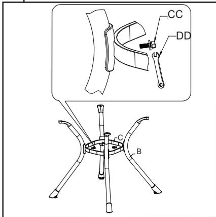
**NOTE: Do not completely tighten bolts until Step 2.**
