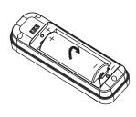
**Step 4:** Rotate battery to make sure it is properly seated in remote pack, double check the battery polarity is correct.
