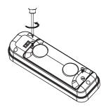
**Step 1:** Loosen screws located on the back of the battery pack.
