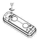
Step 5: Replace cover and tighten screws.
