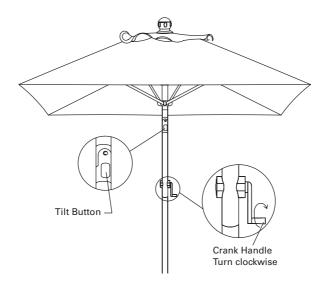
**Step 3:** Turn crank handle in clockwise direction (to right) until canopy is fully opened. Turn crank handle in opposite direction to close canopy and secure with attached strap. To close the umbrella, it must be in the upright position.
