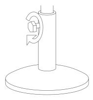
**Step 4:** Insert umbrella into a heavy umbrella base no less than 25.5 lbs (not included). Tighten locking nut on side of base to safely secure umbrella.
