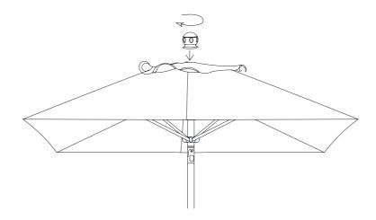
**Step 1:** If not attached, align finial (A) to threading on top of umbrella frame (C) and turn clockwise (to right) to lock into place. Do not over-tighten.
