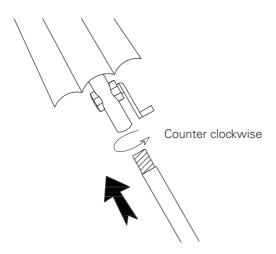
**Step 2:** Attach bottom pole (D) to umbrella frame (C), then tighten in counter clockwise direction.
