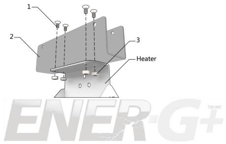
Step 2: Fix the 'U' support to tube.
